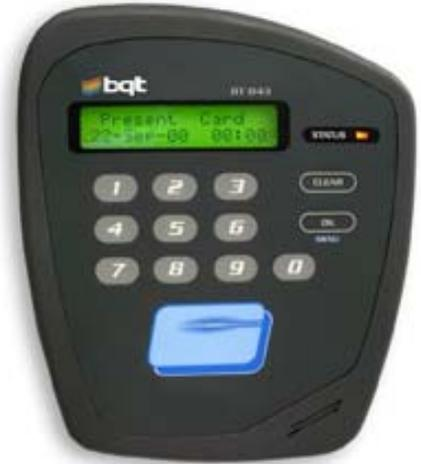
The keypad provides an additional layer of user authentication with the addition of a PIN. The PIN may be stored in the memory of the card and is authenticated by the reader. The reader can be ordered to provide various Wiegand strings output in various formats for retrofitting or for upgrading from a 125 KHz proximity system to Mifare. PIN in the card means that the administrator need no longer manage the individual user PIN. The user defines their own PIN.
